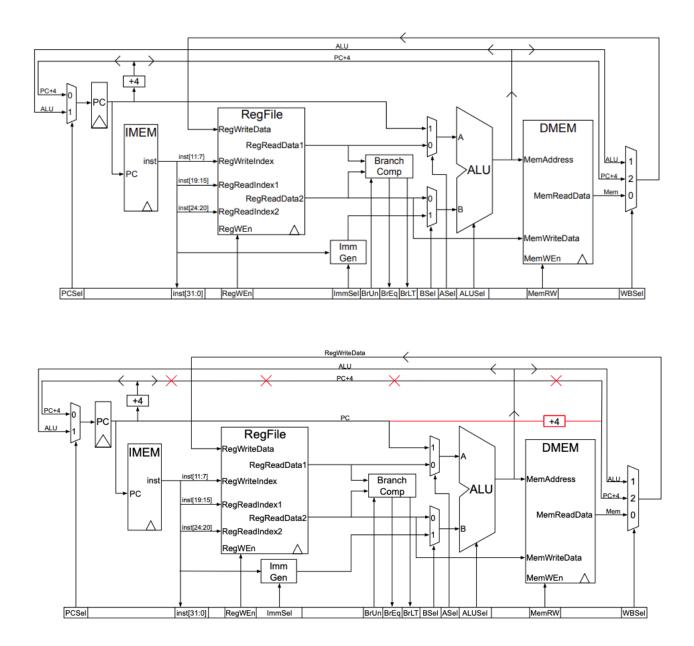
2.1 Two diagrams are provided above. The topmost one is the standard single cycle datapath. The second is a modified version. Compare these two diagrams and explain the difference.
