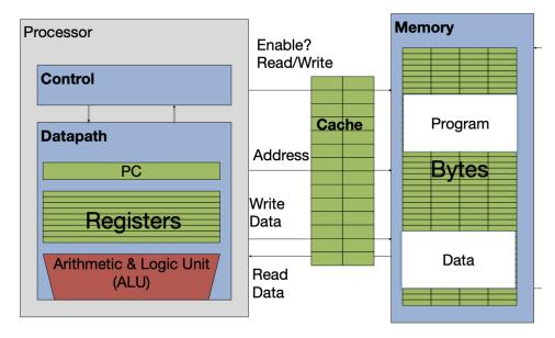
As seen above, the access to cache is the middle step between the CPU asking for a memory bit, and the actual main memory access - if the data is not found in the cache, only then is main memory accessed. This way unnecessary trips to main memory are avoided. One important detail is that caches are much smaller in size than main memory - this is why we have to be efficient in what we hold in caches.
