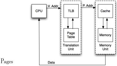
A chunk of memory or disk with a set size. Addresses in the same virtual page map to addresses in the same physical page. The page table determines the mapping.
